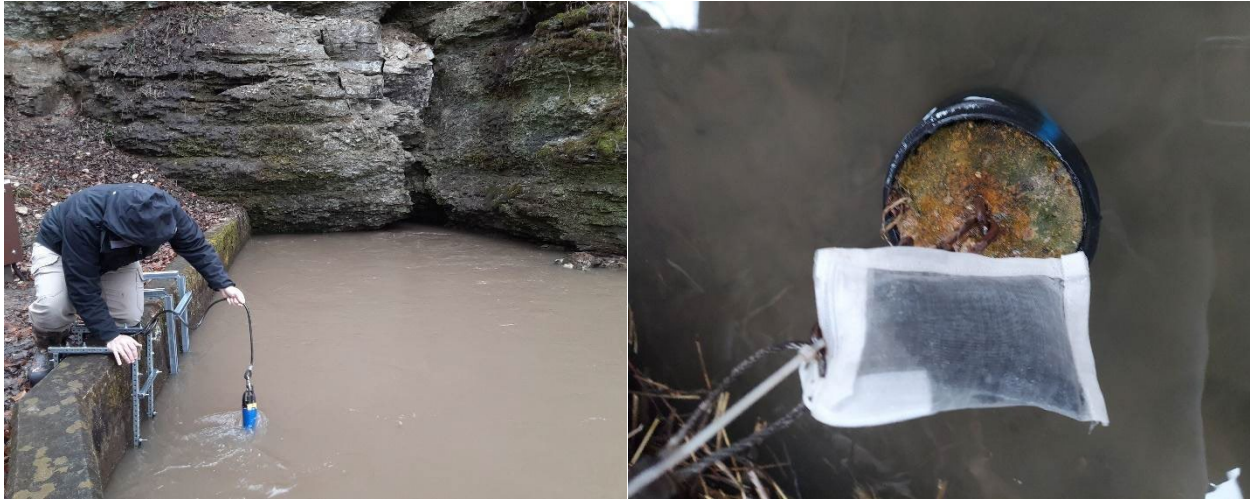
Figure 42. Left: Rhodamine sensor installed at Siewers Spring during Trout Run dye traces. Right: Charcoal packet placed at sites instream and in household toilet tanks during dye trace 1 and 2.
