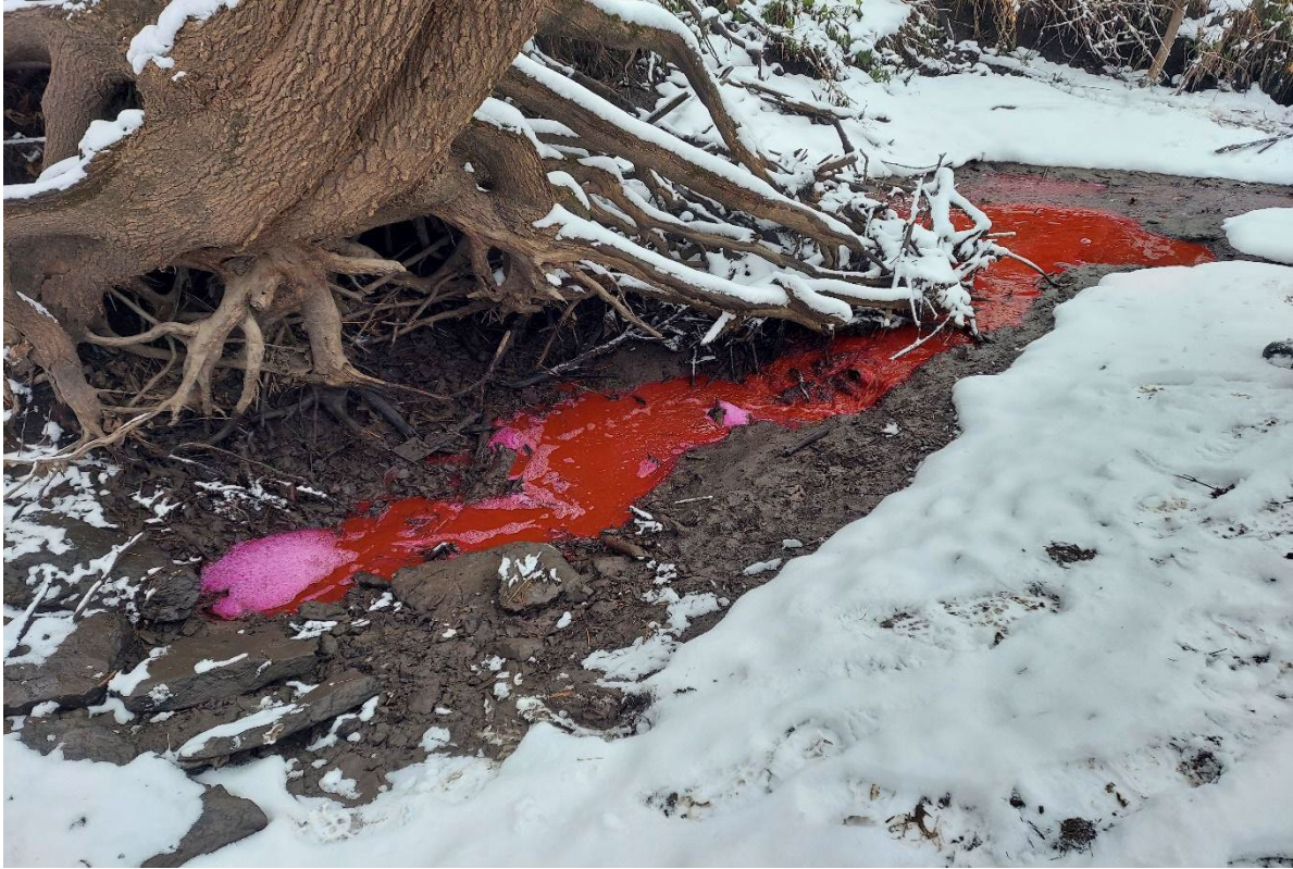
Figure 47. Rhodamine dye flowing into a losing stream reach in the Washington Prairie Branch of the Trout Run watershed. Direction of flow goes from top right to bottom left.
