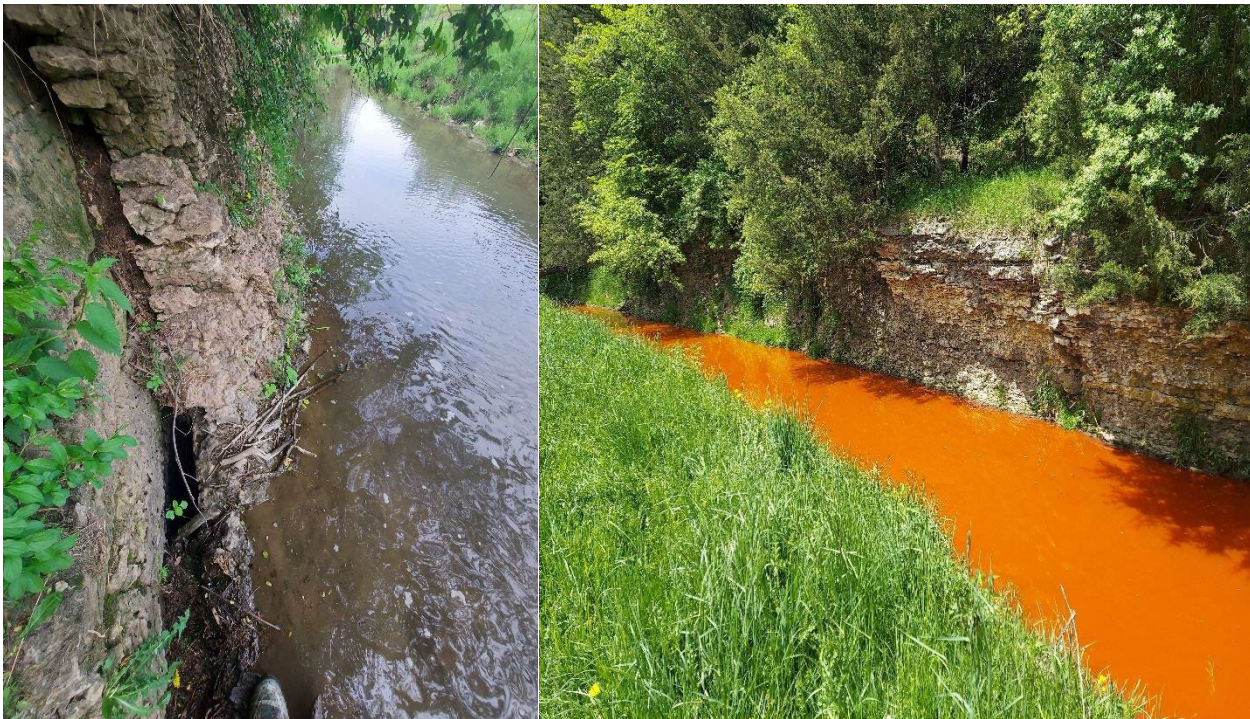
Figure 45. Left: a fracture in the stream bed of a losing stream reach in Trout Creek. Right: dye trace #2 along a losing stream reach on the West branch of Trout Creek.
